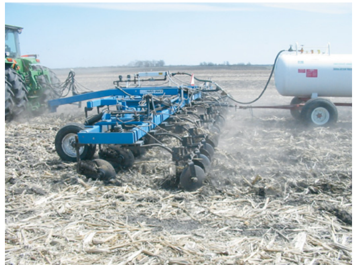
Figure 1. Increased clearance and ability to handle larger amounts of surface residue are common features in newer equipment.
